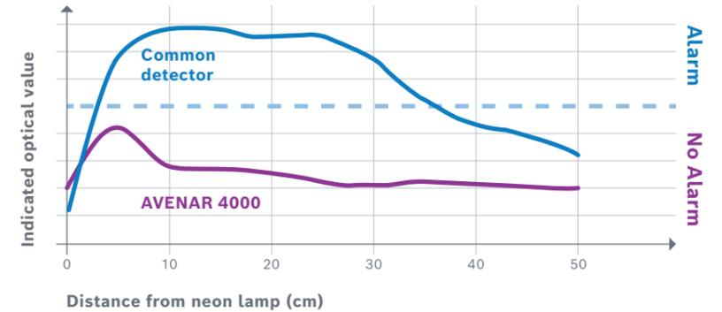
The graph shows the optical value of the detector which varies because of the influence of electromagnetic fields when no smoke is detected (as a function of the distance).
